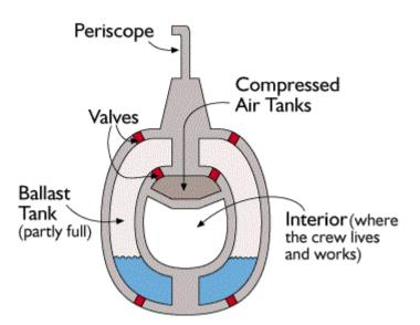
When the **submarine** is at the surface, its ballast tanks are filled with air, thus making its density less than that of the surrounding water. In order to submerge, the ballast tanks are filled with water, making the overall density of the ship higher than the surrounding water
